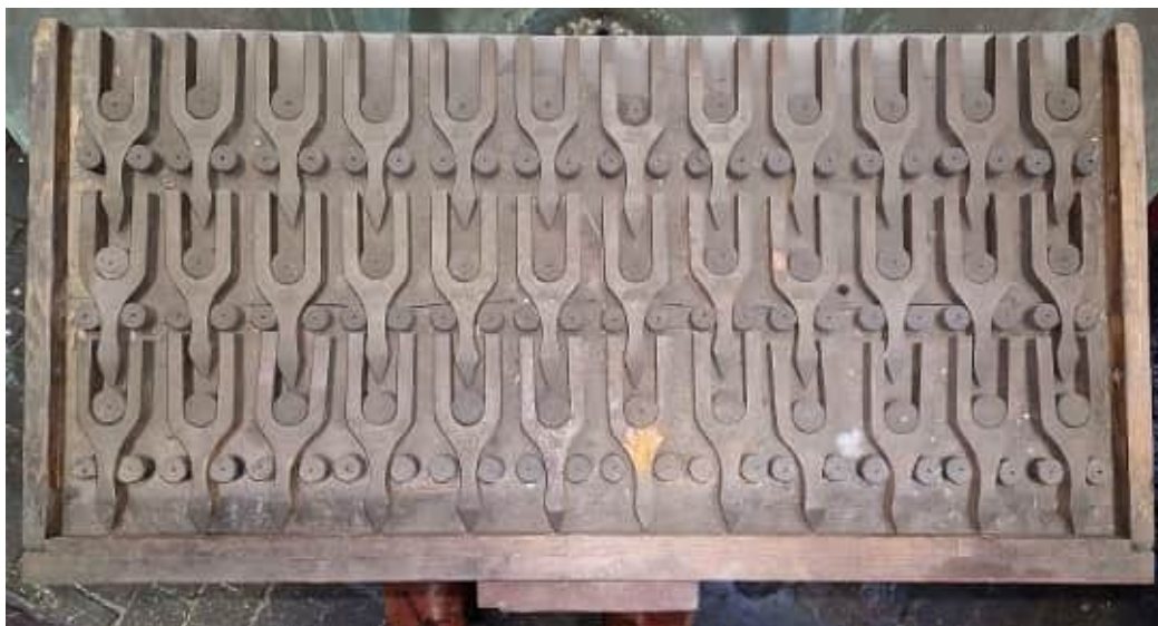
This is a tray of Gillett's forks, covering frequencies 2132Hz to 2272Hz.
